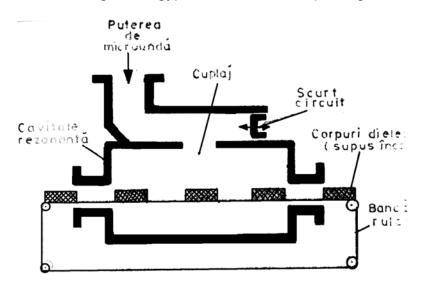
Fig. 2 – The resonant cavity for heating gypsum samples.
