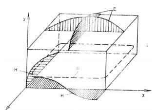
Fig. 1 – The distribution of electrical fields E and magnetic fields H in the paralelipipedical cavity.
